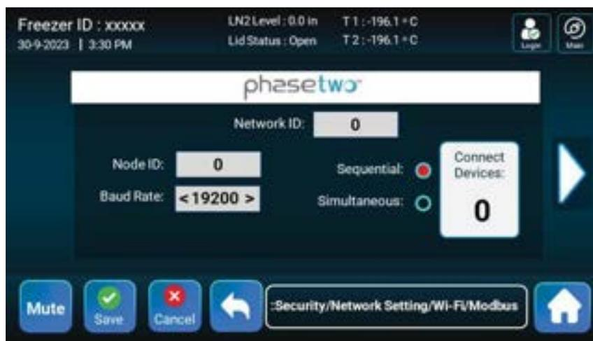
First create a network ID. This value can be up to 8 characters and must be only numbers and letters. No spaces are allowed. Next set the master unit node ID to 0 and press the Save button. Note: The Save button must always be pressed after
