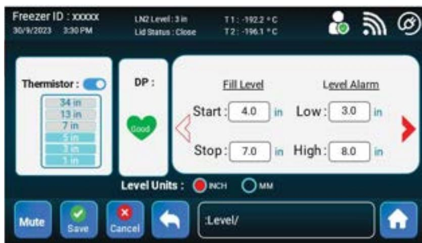
At first glance of the level menu, you get a quick status view of the DP and which thermistors are submerged in LN2. As explained in the operation menu the
