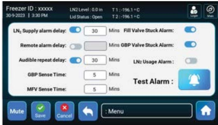
The alarm submenu is used to configure all alarms excluding lid related alarms. Below is a detailed description of each option.
