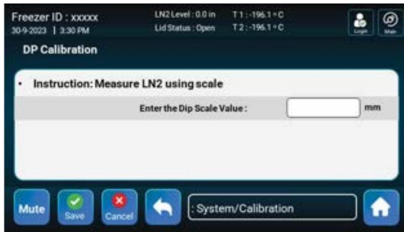
To complete a DP calibration simply measure the DP height as close as possible to the center of the tank with the manual dip stick provided with the tank. To manually measure liquid level, dip the dipstick in the tank for 5 to 10 seconds, pull the stick out and wave it in the air. A distinct frost line will occur. Subtract 0.5" from the frost line to account for liquid boiling during the measurement.
