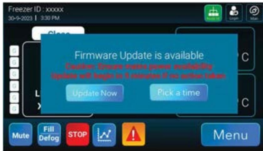
Either configure an update time or select update now. Note: The 'pick a time' option cannot exceed more than one week. The unit will say "Firmware updating please do not disconnect from power". The unit will boot normally once the firmware update is complete.
