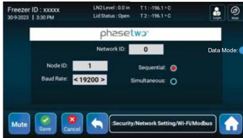
Once the unit is configured, the below tables explain the mapping structure of the data. Note: All available data is in Modbus RTU holding registers.
