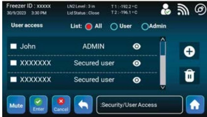
A total of 10 user accounts (2 Admin users and 8 Normal users) can be created in the database. Normal users can access all submenus and settings in menus except security submenu. Admin users have full access to all submenus including security submenu.
