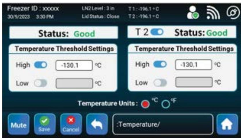
T1 cannot be disabled. T2 can be disabled. The status of the RTD's is either good or open. Open could mean that no RTD is plugged in, or it is defective. To enable the Low Temp alarm, select the toggle next to Low, click in the textbox area, and type a value. For any changes to be saved you must hit the Save button before leaving the menu. All temperature alarms can be disabled. It is not recommended that the High Temp alarm is ever disabled other than on the first fill.
