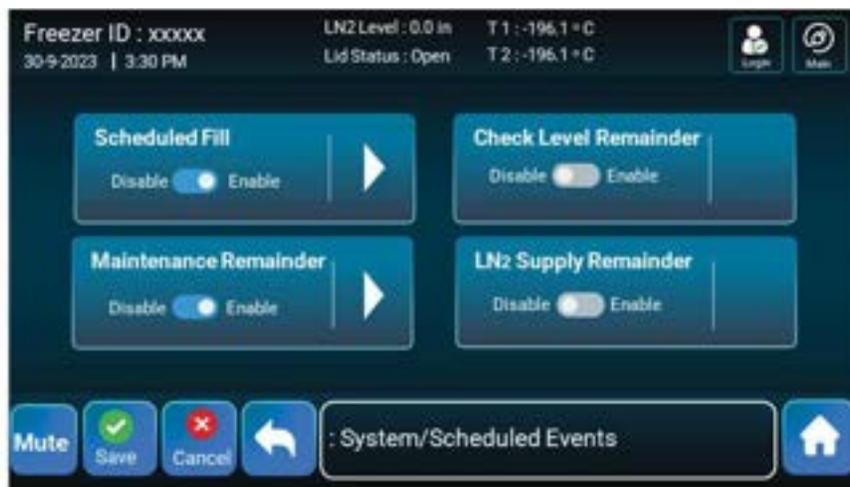
On this menu you can set up a Scheduled Fill, Maintenance Reminder, Check Level Reminder, and LN2 Supply Reminder. To enable one simply toggle the switch to Enable and click Save. Then click the arrow next to it to configure further.
