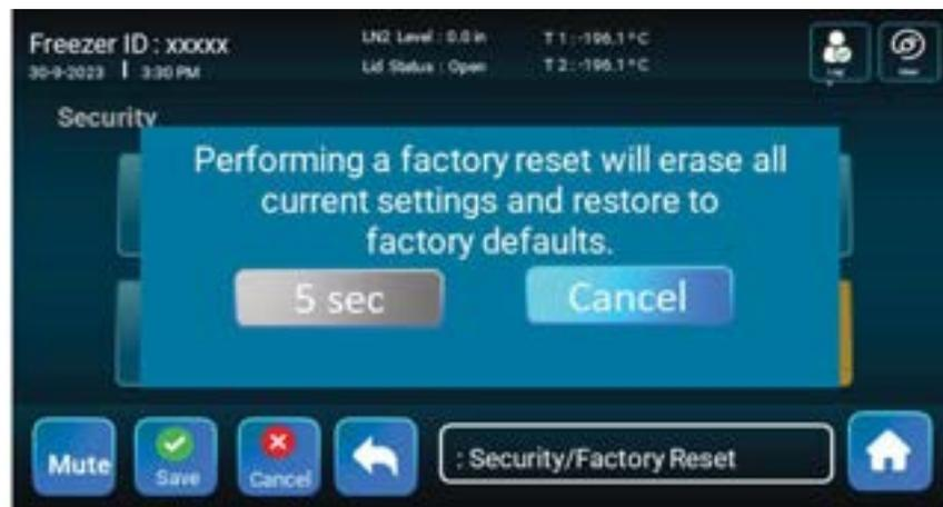
A delay of 5 seconds is implemented before a factory reset is done to ensure the user intentionally reset the settings.
