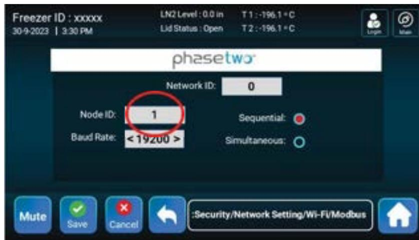
Note: Please ensure that each freezer is assigned a unique node ID (from 0 to 31). Also please ensure that there is 1 master. Duplication of IDs will result in malfunctioning of network.
