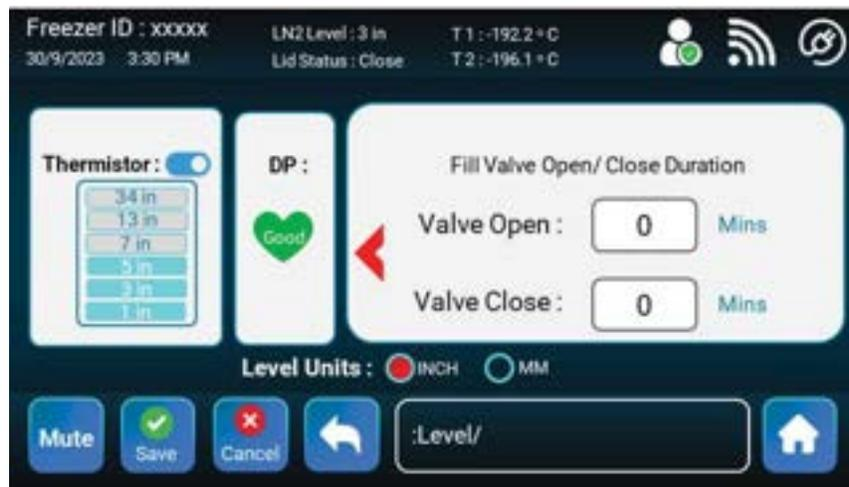
If turning the valve On & Off in a pulsed manner is required, adjust the Valve Open and Closed times accordingly here.
